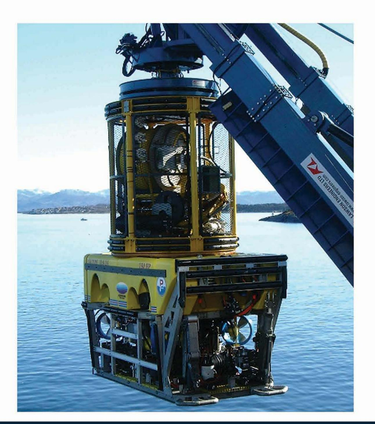
Deep-water operations are aided by the use of a complimentary top hat tether management system (TMS), designed to maximise the performance of the vehicle by eliminating the effects of umbilical drag and vessel motion.
