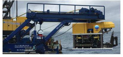
With a depth rating of 300 meters that covers most areas of operation that is feasible with a free flying ROV without pushing the limits.
