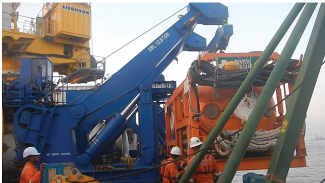
Demonstration of HRC Launching
