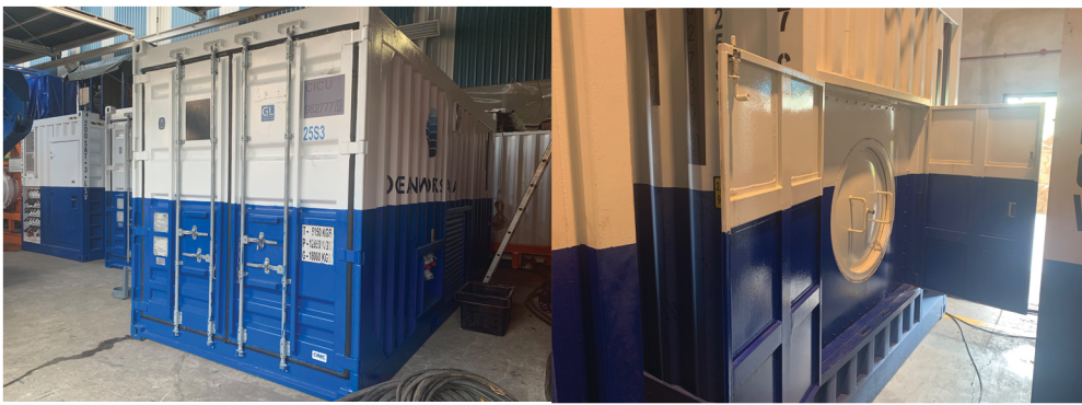
Combined Dive Control and DDC Container
