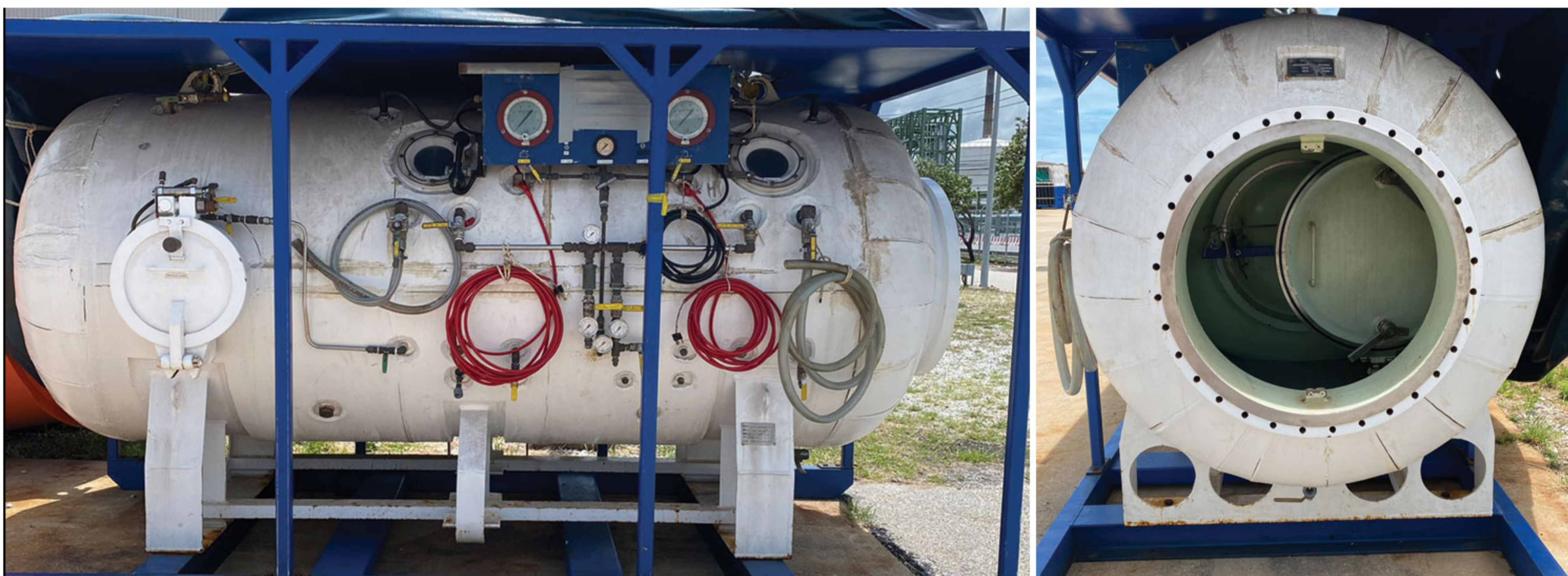
Deck Decompression Chambers (D.D.C.)
