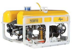
The Seaeye Tiger is widely regarded as the leading observation vehicle within the oil and gas industry. Increasingly they are also being taken up as the ROV of choice by clients seeking increased capability in deep water.
